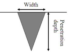
Figure 2: Weld nugget dimensions produced by spot laser welding.
