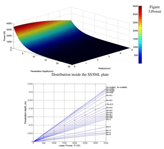
Figure 4: Penetration depth versus laser power
